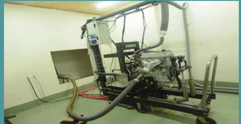
Figure 1: Superflow dynamometer for testing automobile engines
