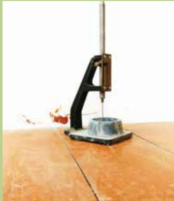
Name: Vicat apparatus Brand: ELE, UK Test Capabilities: To determine the setting time of cement
