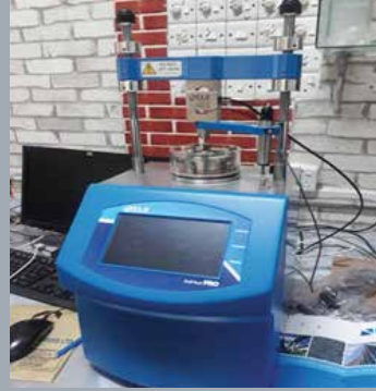
Name: Auto Soils Consolidator (ASC) Brand: ELE, UK Test Capabilities: To measure the pre-consolidated pressure of the soil.
