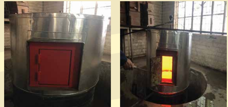
Figure 11: Fire chamber for testing fire resistant door
