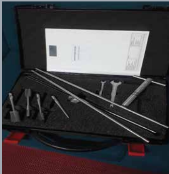
Name: Field Vane Shear Tester Brand: ELE, UK Test Capabilities: To measure the shear strength of soil.
