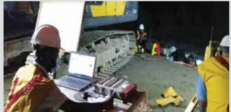
Figure 10: Data collection using Linear Variable Differential Transformer (LVDT) for plate load test of MRT
