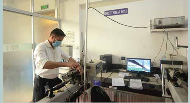
Angle of internal friction of cohesion-less soil is being carried out by Direct Shear Machine at Geo-technical Engineering Lab of CATS-MIST (CE)
