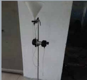
Name: Pinhole Apparatus Brand: Controls, USA Test Capabilities: To evaluate the erodibility of clay soils by flowing water through a small hole that is drilled through the compacted specimen.
