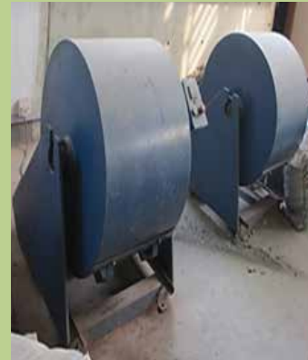
Name: Los angeles abrasion machine Brand: ELE, UK Test Capabilities: To perform abrasion test
