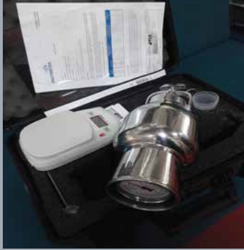
Name: Field Moisture Content Tester Brand: ELE, UK Test Capabilities: To measure the moisture content of soil at field conditions.
