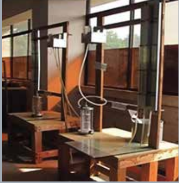
Name: Permeameter Brand: ELE, UK Test Capabilities: To measure the water passing capacity of the soil for the design of embankment.
