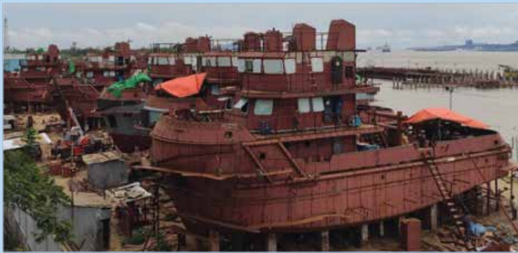
Figure 5: Construction work of Tug Boats in Karnafuly Dockyard, Chattogram
