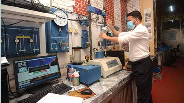
Shear strength of soil is being carried out by Tri-axial Machine at Geo-technical Engineering Lab of CATS-MIST (CE)
