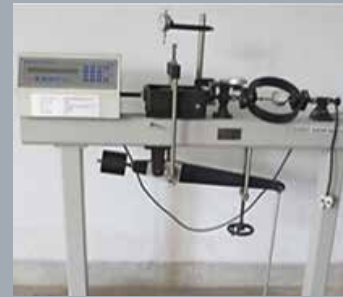
Name: Direct Shear Test Machine Brand: ELE, UK Test Capabilities: To measure the frictional angle of the soil.
