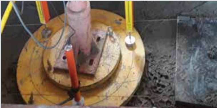
Figure 10: Data collection using Linear Variable Differential Transformer (LVDT) for plate load test of MRT
