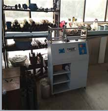
Name: Horizontal Automated Extruder Brand: COOPER, USA Test Capabilities: To be used for the extraction of undisturbed soil.
