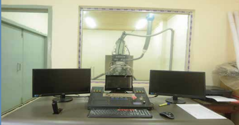
Figure 2: Dynamometer control unit
