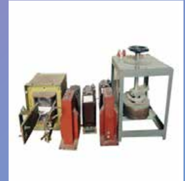
CT/PT test with variac & current injector.
