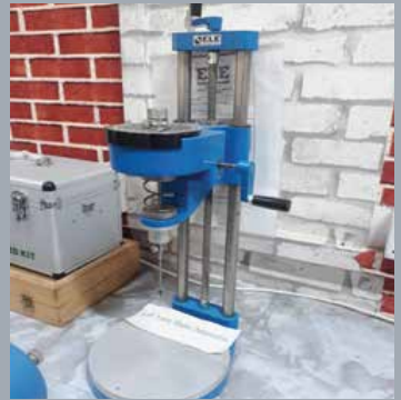
Name: Lab Vane Shear Apparatus Brand: ELE, UK Test Capabilities: To measure the shear strength of soil.
