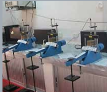
Name: Consolidation Apparatus Brand: ELE, UK Test Capabilities: To measure the pre-consolidated pressure of the soil.
