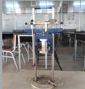
Name: Moisture Conditioning Value Apparatus Brand: ELE, UK Test Capabilities: To measure moisture content of the soil.
