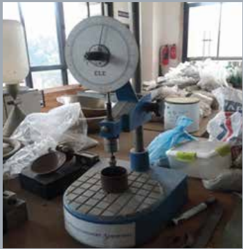
Name: Cone Penetrometer Brand: ELE, UK Test Capabilities: To measure the liquid limit of the soil.
