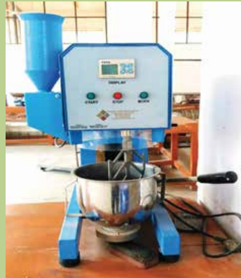
Name: Mortar mixer machine Brand: Local brand Test Capabilities: Mixing the concrete
