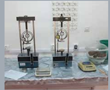
Name: Unconfined Compression Test Machine Brand: ELE, UK Test Capabilities: To measure the Cohesion of the soil.
