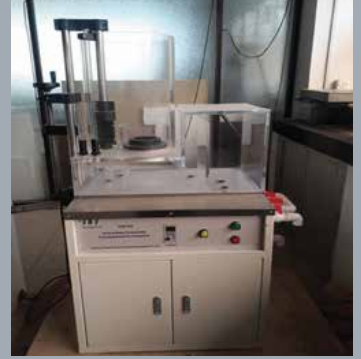
Name: Vertical Permeability Apparatus Brand: TBT, China Test Capabilities: To measure the permeability of the geotextiles.
